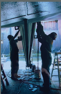
ON THE COVER Shipyard workers attach chain hoists beneath Arni J Richter hull in dry dock. This is the smallest of all the Bay Ship dry docks, and was utilized in the early days of the original Bay Shipbuilding - Drydock company.
