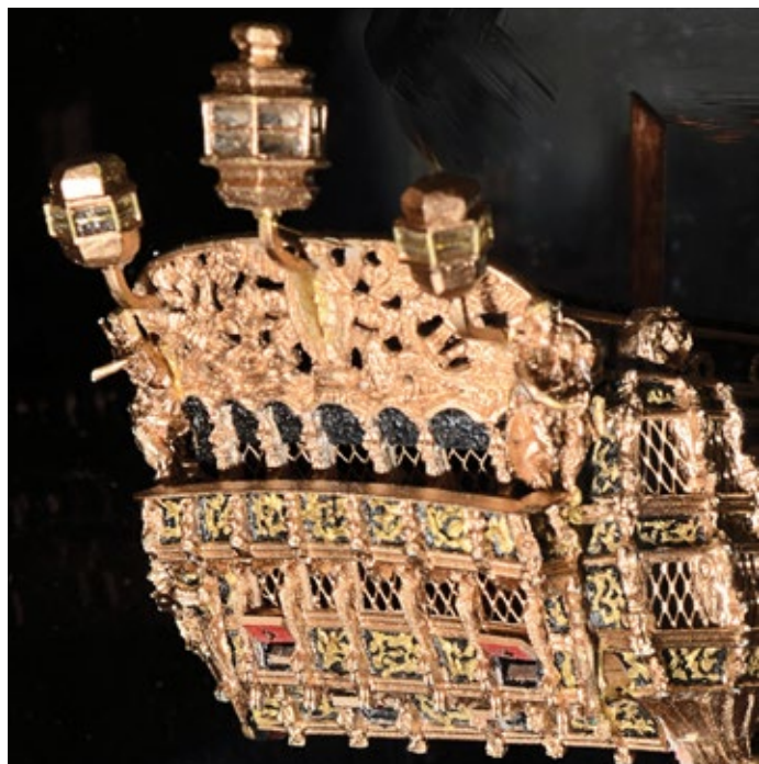
More than 50 gold-painted boxwood carvings adorn the stern of Gus Agustin's HMS Sussex (1693) at 1/16 inch equals 1 foot (1:192) scale. Windows were drilled out, then cleaned up with an X-Acto knife and square needle file.
